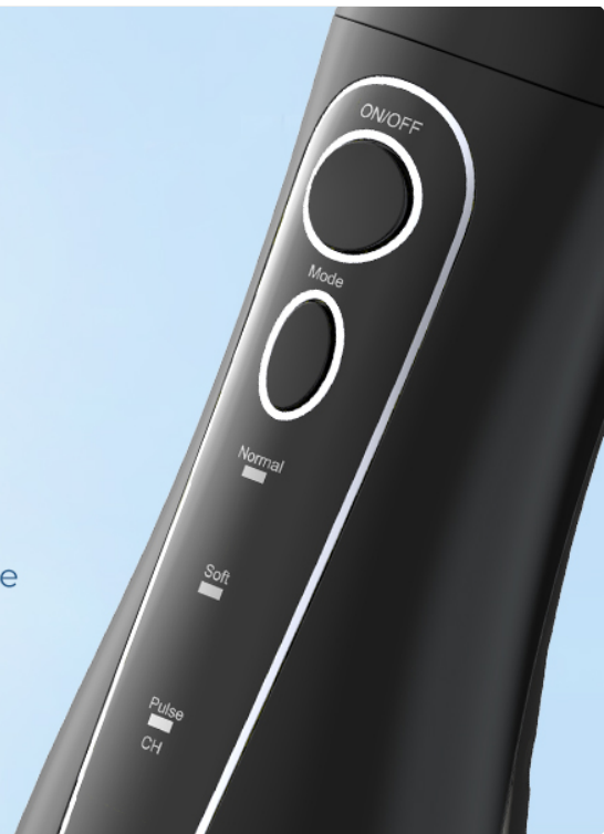
Image: The control panel of the water flosser, highlighting the three operational modes.
