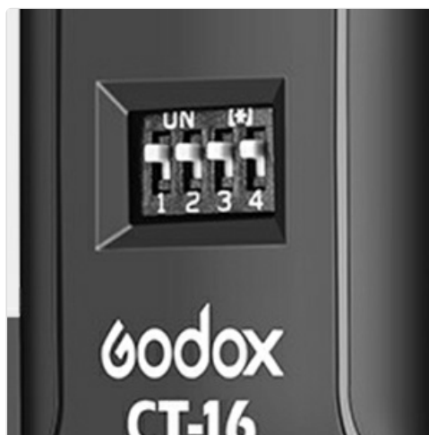
Image 3.2: Close-up view of the transmitter's channel DIP switches.
