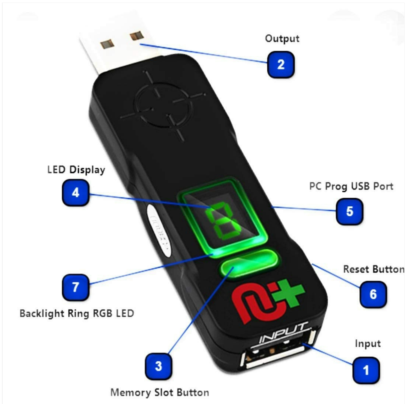
Image: A detailed diagram of the CronusMax Plus device, with key components labeled for easy identification.
