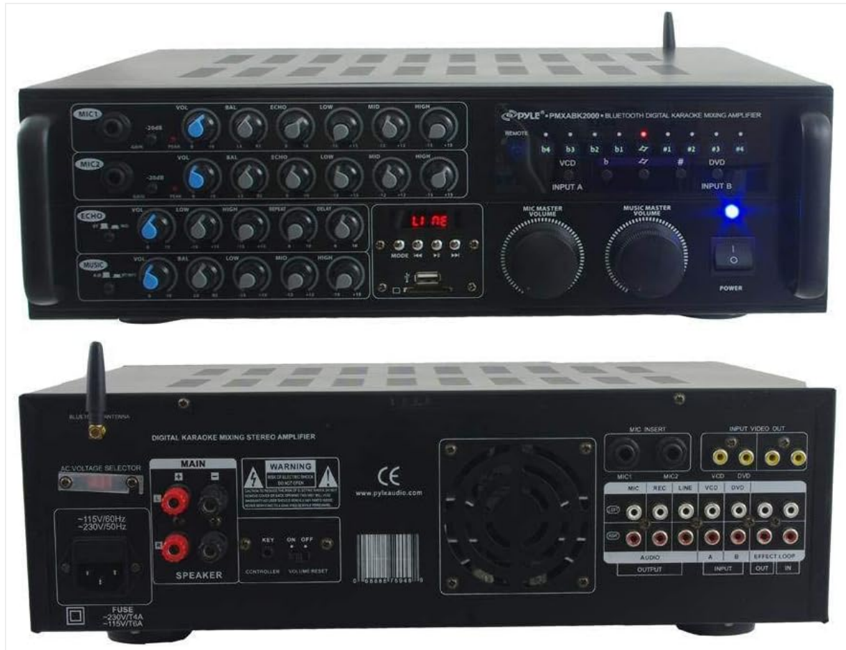
Figure 4.2: Rear view of the amplifier, highlighting speaker outputs, audio inputs/outputs, video inputs/outputs, and microphone insert jacks.
