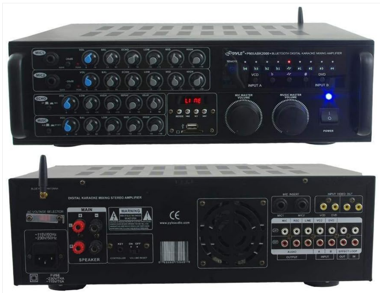
Figure 5.1: Speaker output terminals on the rear panel, compatible with banana clips and bare wire.
