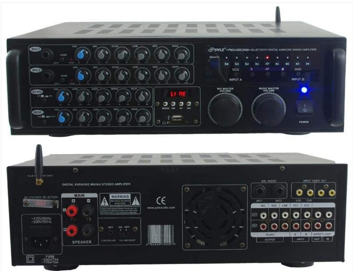
Figure 4.1: Front view of the amplifier, detailing microphone inputs, echo controls, music controls, and master volume
