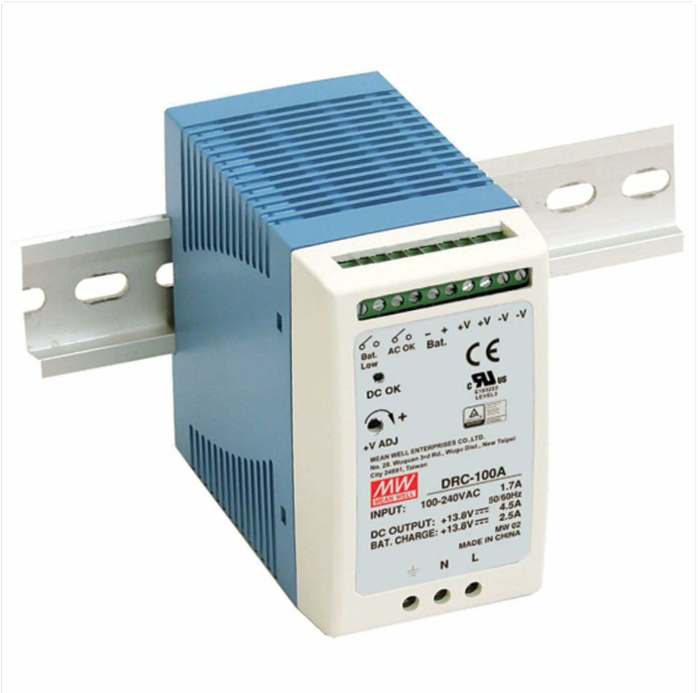
Figure 2: Detail of the DRC-100A front panel showing input terminals (N, L), DC output terminals (+V, -V), battery terminals (Bat.+, Bat.-), alarm signal terminals (Bat. Low, AC OK, DC OK), and the '+V ADJ' potentiometer for voltage adjustment.
