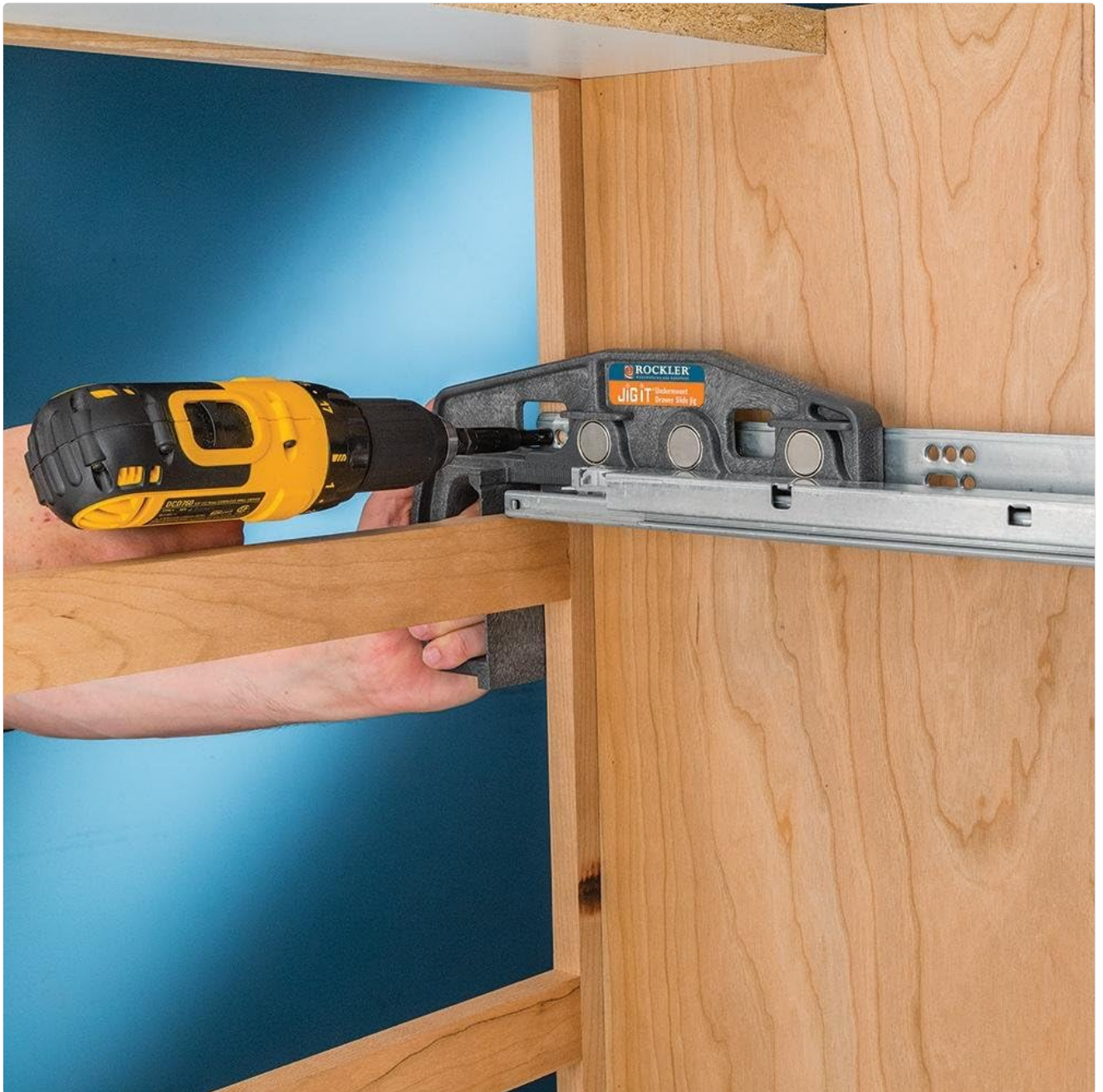
Image: The jig holding a drawer slide in place against the cabinet, ready for screw installation.
