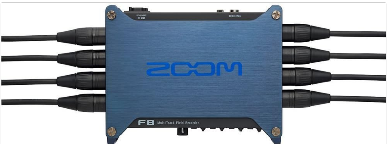
Figure 5: XLR cables connected to the F8 inputs.
