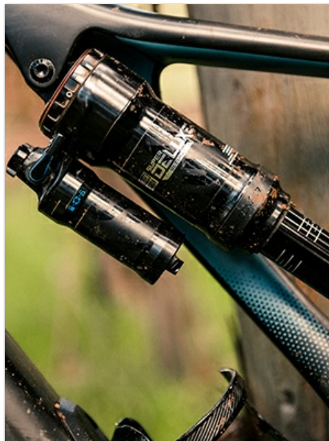
Image 3.1: The Monarch Plus RC3 rear shock properly installed within a bicycle frame.
