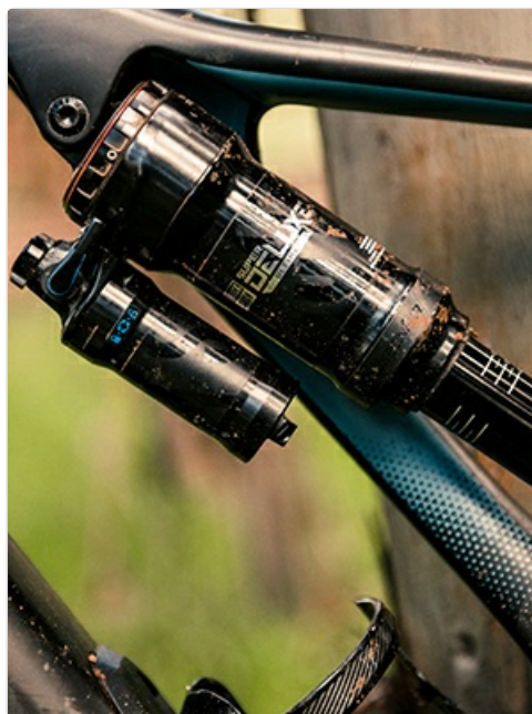
Figure 3: Monarch Plus RC3 installed on a bicycle.
