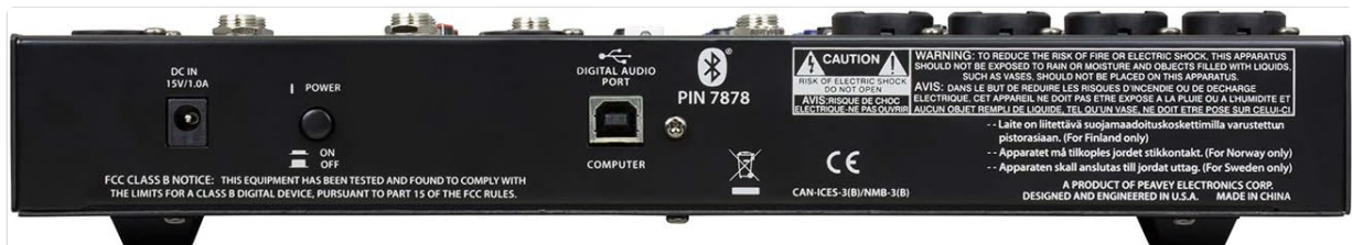
Figure 4.1: Rear panel of the Peavey PV 10 BT Compact Mixer, showing power input, USB ports, and safety warnings.
