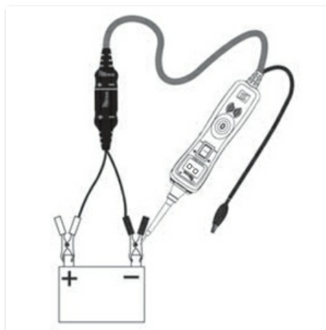
Figure 5.1: Example of using the Power Probe III to test a circuit.
