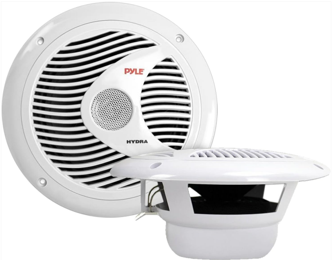
Figure 3.2: A pair of 6.5-inch marine speakers.
