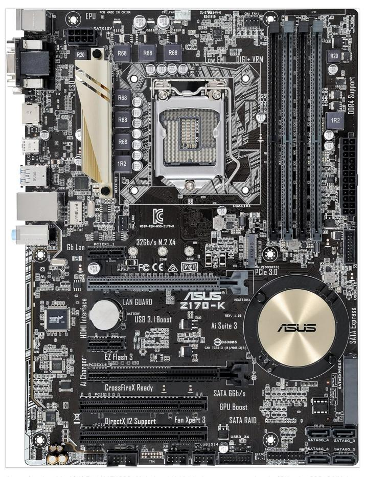
Image: Overview of the ASUS Z170-K ATX DDR4 Motherboard, highlighting key components such as the CPU socket, DDR4 DIMM slots, PCIe slots, SATA ports, and various headers.
