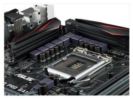
**Image Description:** A close-up view of the LGA1151 CPU socket on the ASUS Z170 PRO Gaming motherboard. The metal load plate is open, revealing the pins within the socket. The surrounding area shows power delivery components and heatsinks, indicating the robust design for CPU stability.
