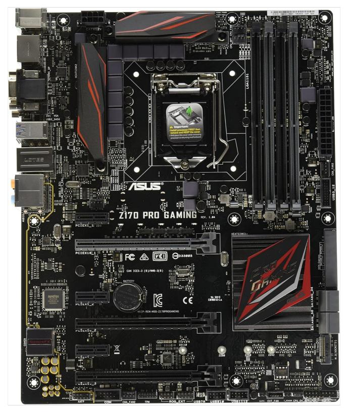
Image Description: This image displays a top-down view of the ASUS Z170 PRO Gaming motherboard. Key components visible include the LGA1151 CPU socket at the center, four DDR4 DIMM slots to its right, multiple PCIe expansion slots below the CPU, and various headers and connectors around the board's perimeter. The I/O panel is visible on the left edge, and the Z170 chipset
