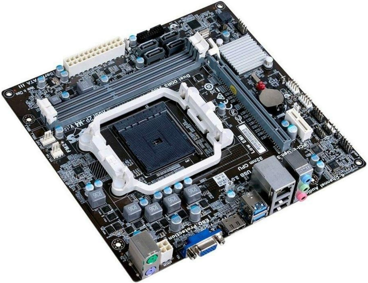
Image 4.2: An angled view of the ECS Elitegroup A68F2P-M4 motherboard, highlighting the CPU socket and DIMM slots.
