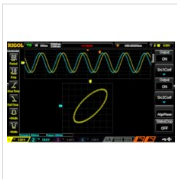
Lissajous figures for phase analysis.
