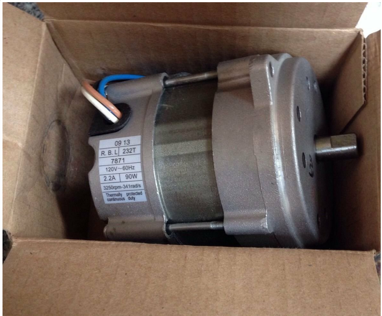
Figure 1: Riello 3005843 Motor in Packaging. The motor's label displays specifications such as voltage, amperage, wattage, and RPM.
