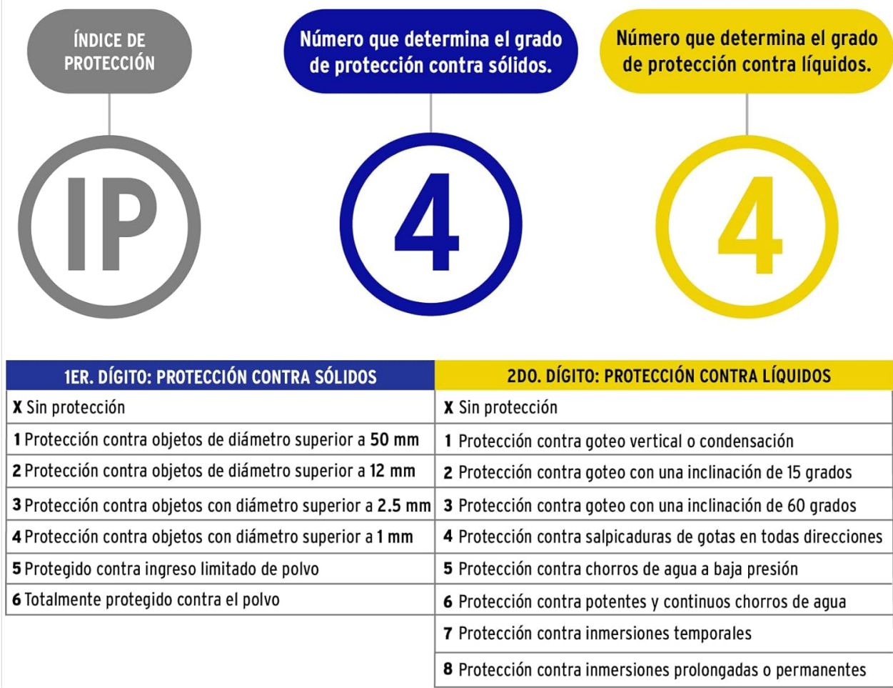
Figure 3: IP (Ingress Protection) Rating. The light has an IP44 rating, meaning it is protected against solid objects larger than 1mm and splashing water from any direction, making it suitable for outdoor use.
