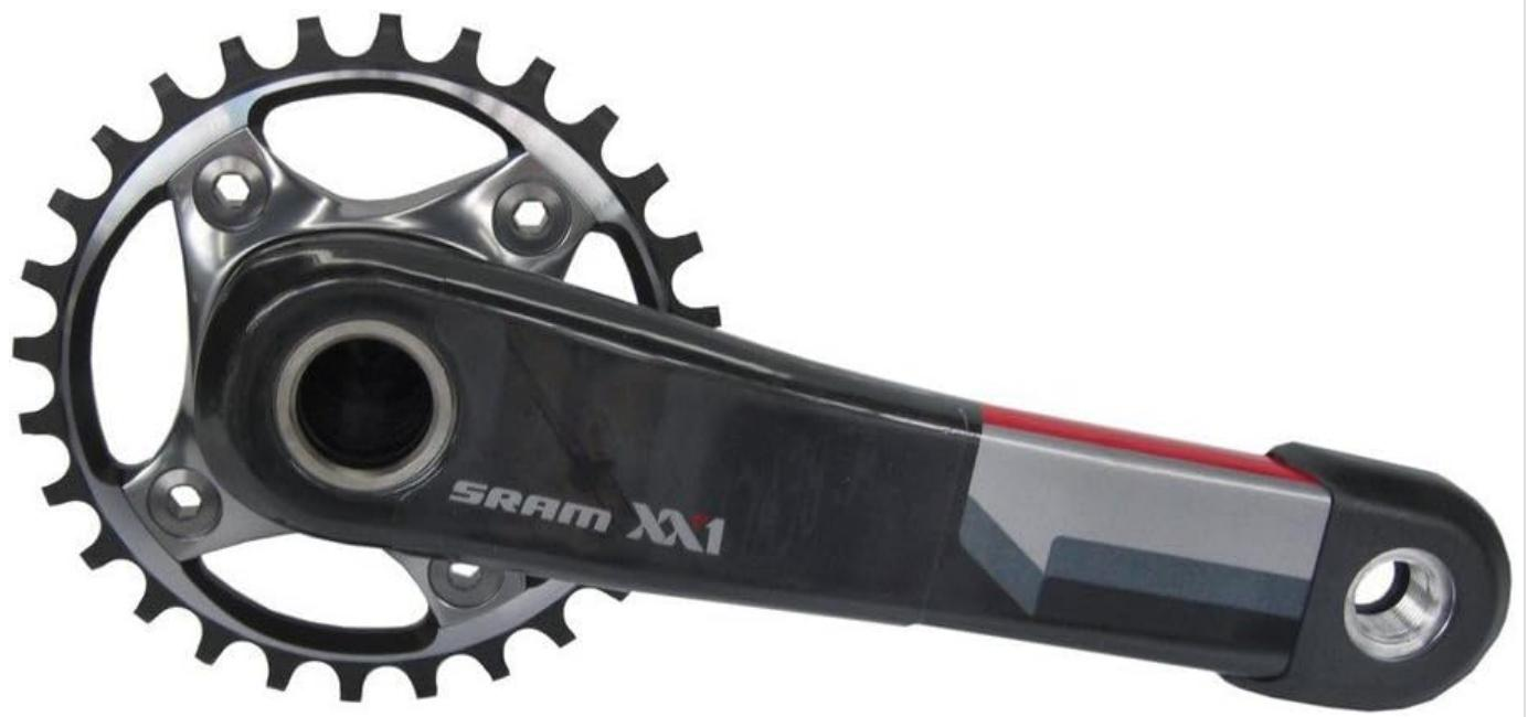
This image displays the SRAM XX1 Fat Bike Crankset, featuring a black carbon crank arm with red and grey accents, and a silver X-SYNC chainring with precisely machined teeth.
