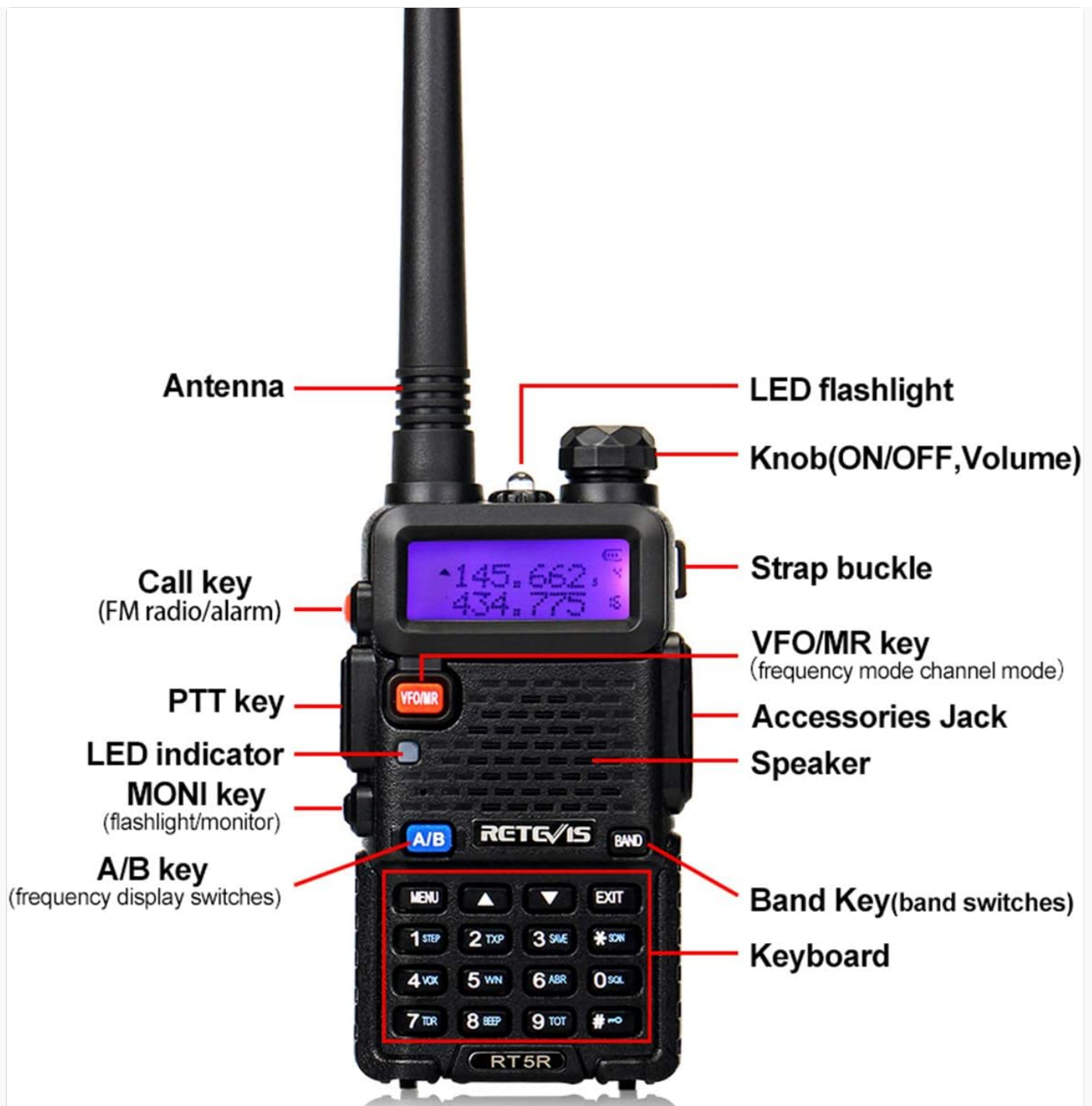
Image: Detailed diagram illustrating the various parts and controls of the Retevis RT5R radio, including the antenna, LED flashlight, knob (ON/OFF, Volume), strap buckle, VFO/MR key, PTT key, LED indicator, accessories jack, speaker, MONI key, A/B key, Band key, and keyboard.
