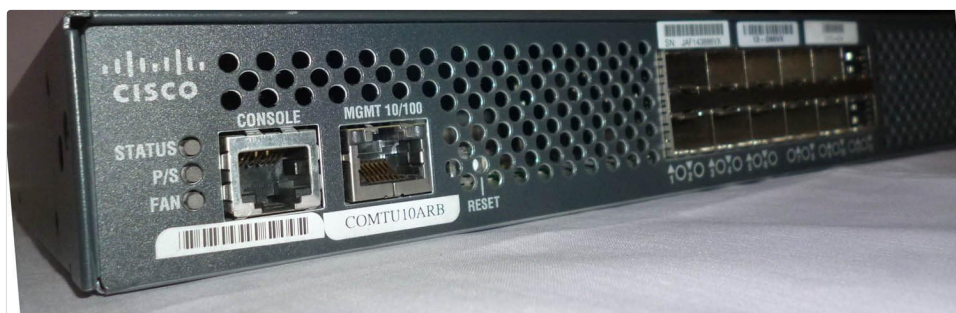
Image Description: A detailed view of the first 12 SFP ports (1-12) on the front panel of the Cisco switch, showing the empty slots for transceivers.
