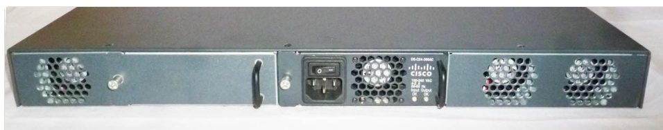
Image Description: A full rear view of the Cisco DS-C9124-K9 switch, displaying the power input module with an AC inlet and power switch, along with multiple fan exhaust vents.
