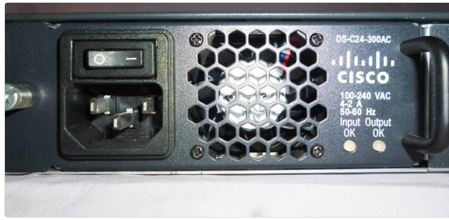
Image Description: A close-up of the power input module on the rear panel, showing the AC power inlet, the power switch, and the "DS-C24-300AC" label, along with input/output OK LEDs.
