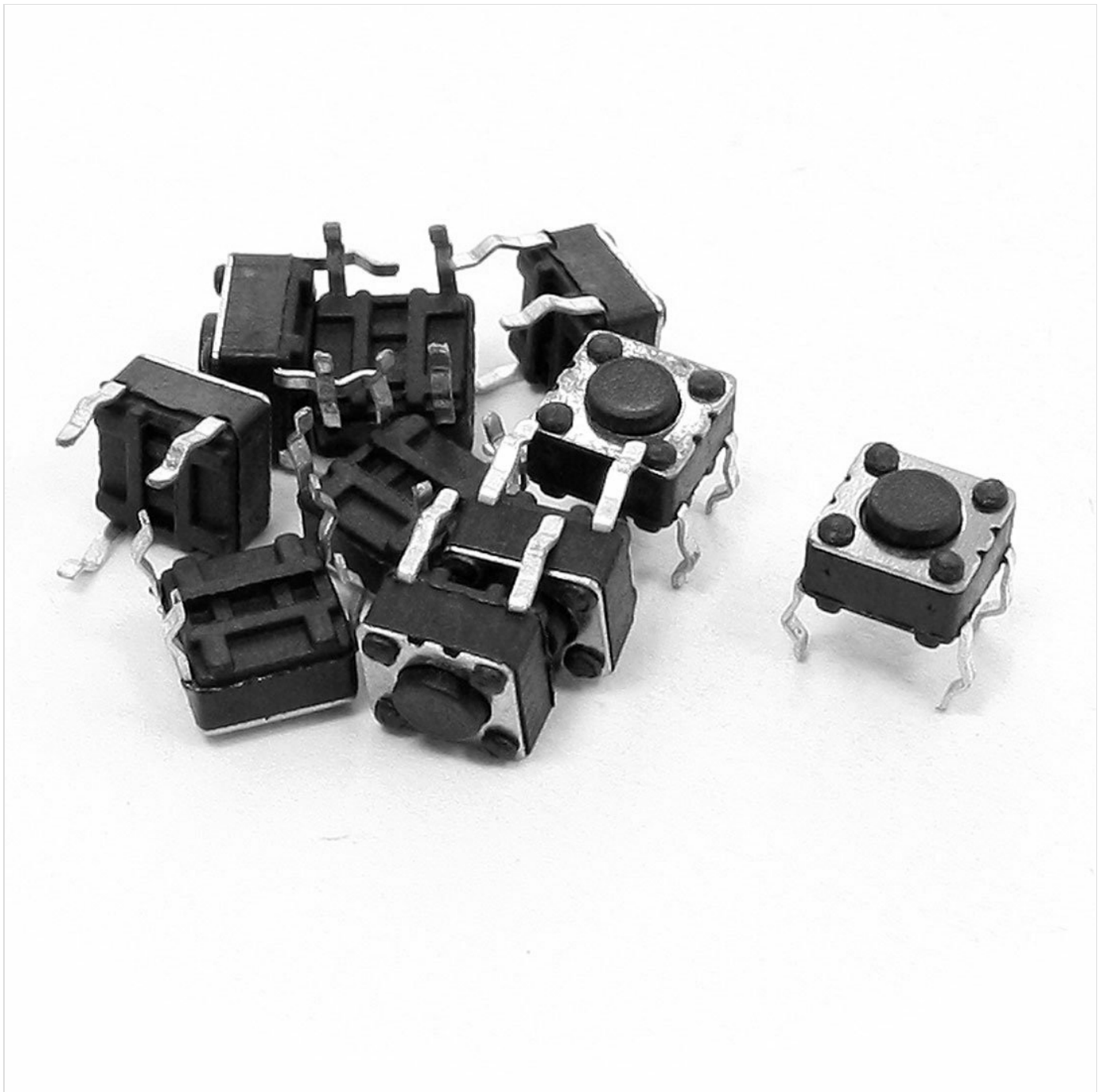
Figure 2.1: A collection of Uxcell 4-pin momentary tact push button switches, showing their compact size and pin configuration for PCB mounting.
