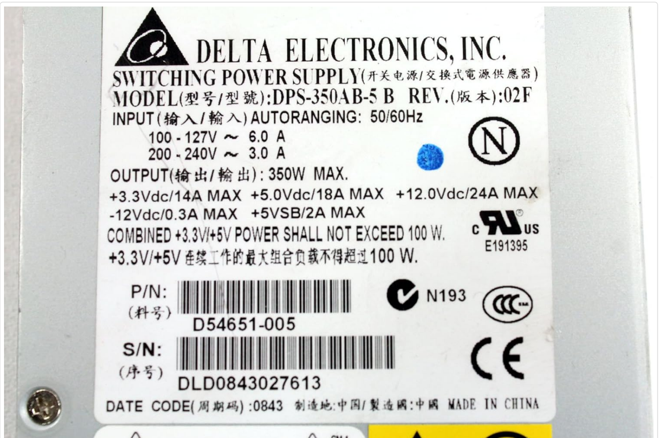
Detailed view of the product label, displaying model number DPS-350AB-5 B, part number D54651-005, serial number
