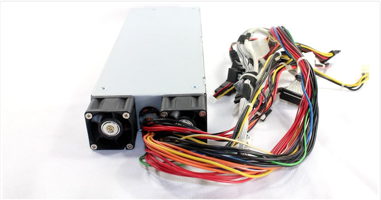
Rear view of the power supply, highlighting the dual cooling fans and the bundled output cables.
