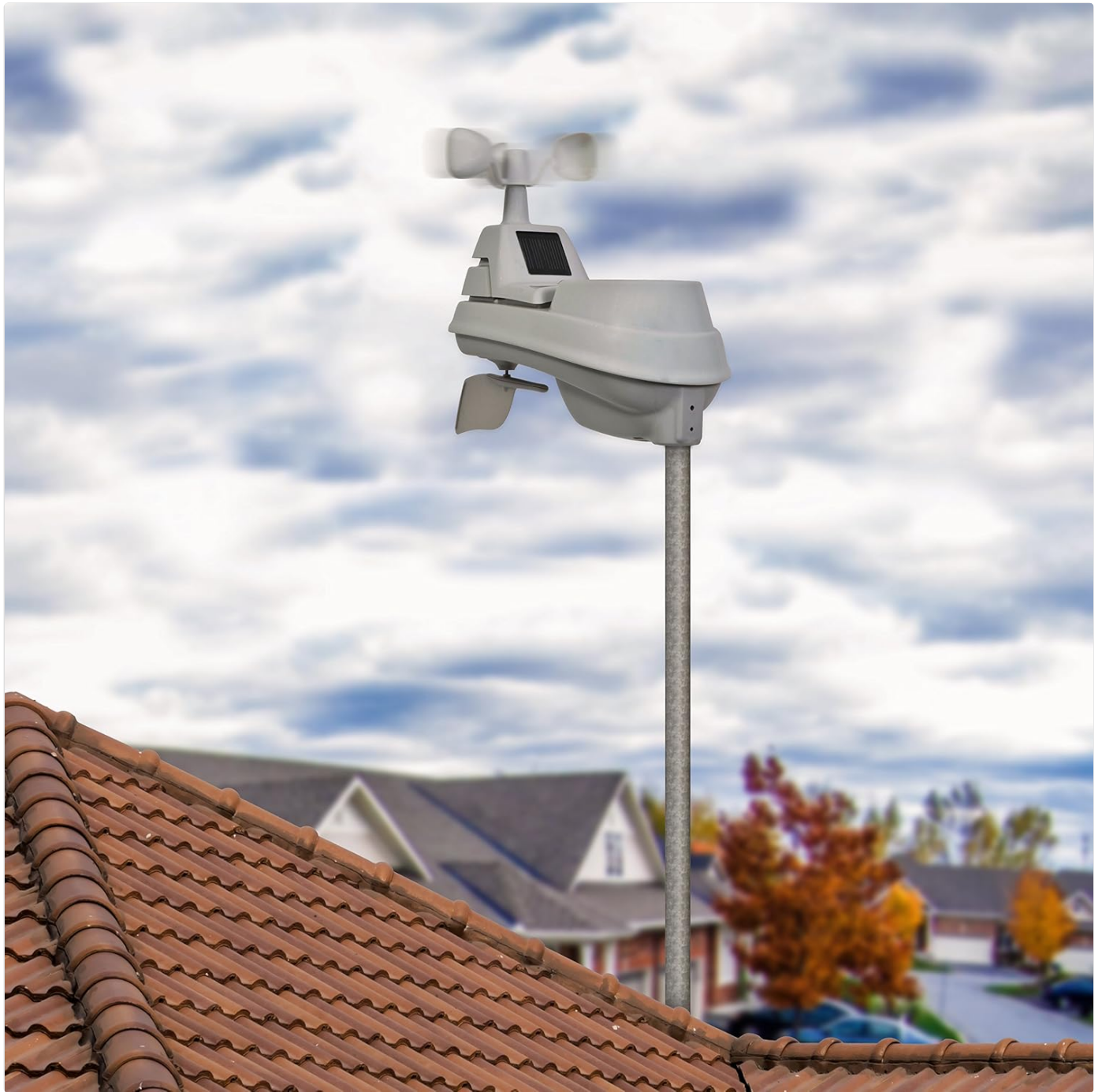
Image 3.1: The 5-in-1 wireless sensor correctly mounted on a pole, elevated above the roofline for optimal data collection.
