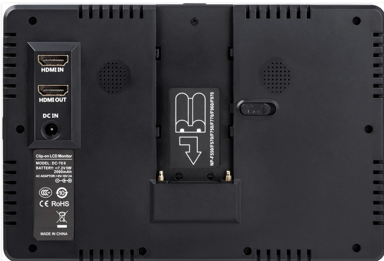
Image: Rear view of the VILTROX DC-70 II Field Monitor, highlighting HDMI In/Out, DC In, and the battery plate.
