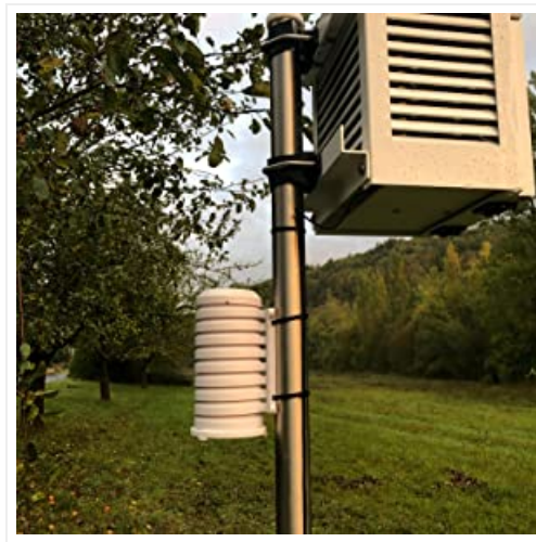
Image: Optional TFA Dostmann 98.1114.02 Weather Protection Housing, which can be used to protect the sensor from direct rain and harsh weather conditions.
