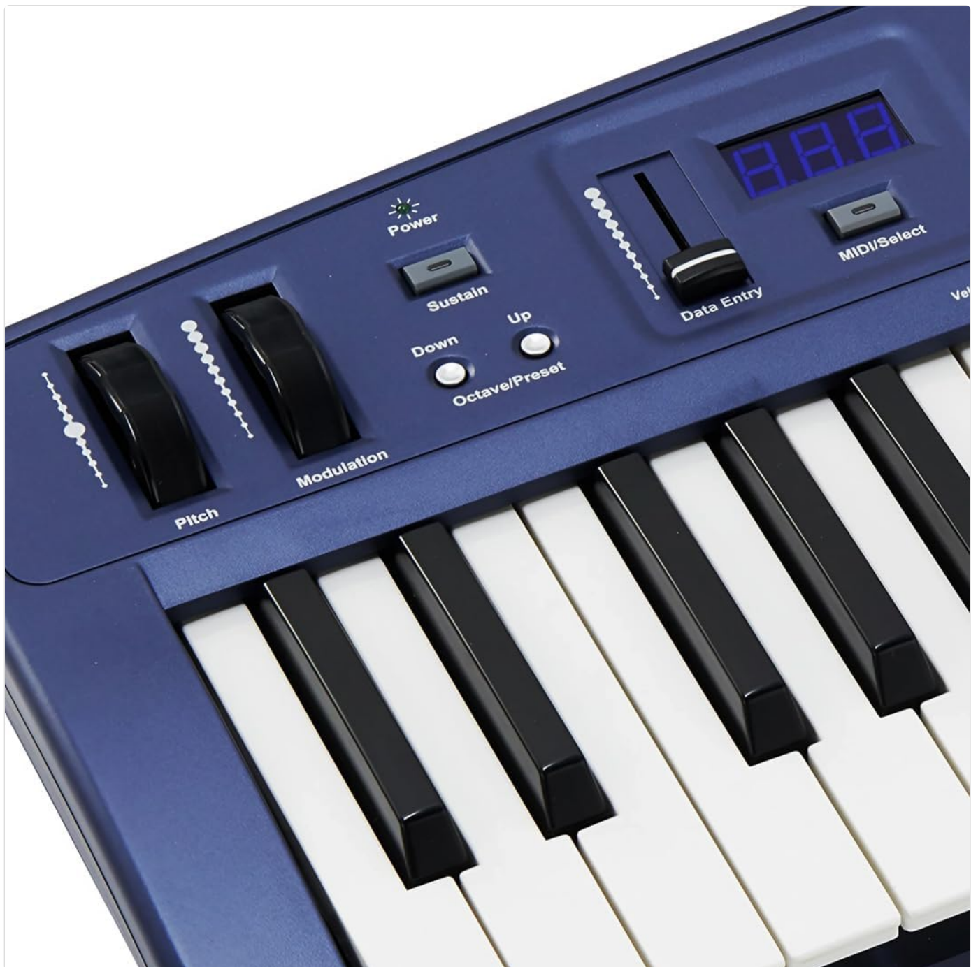
Figure 4.2: Detail of the left-side controls, including Pitch Bend, Modulation, Power, Sustain, Octave Up/Down, Data Entry slider, and LED display.
