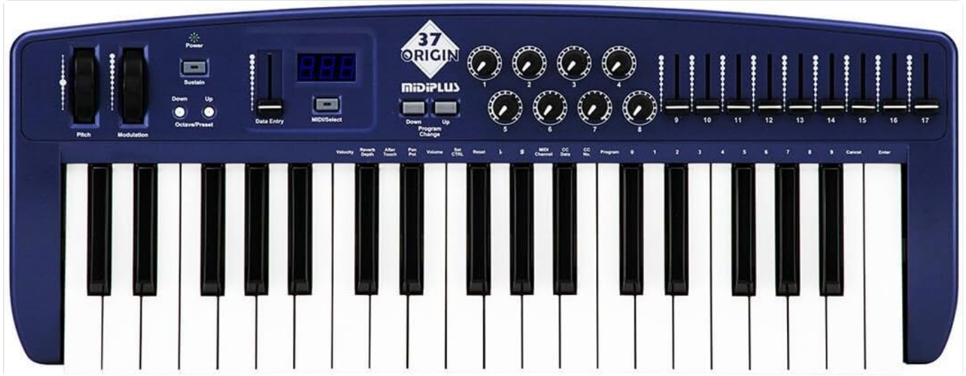
Figure 4.1: Top-down view of the midiplus Origin 37, showing the 37 keys, pitch and modulation wheels, control knobs, sliders, and display.
