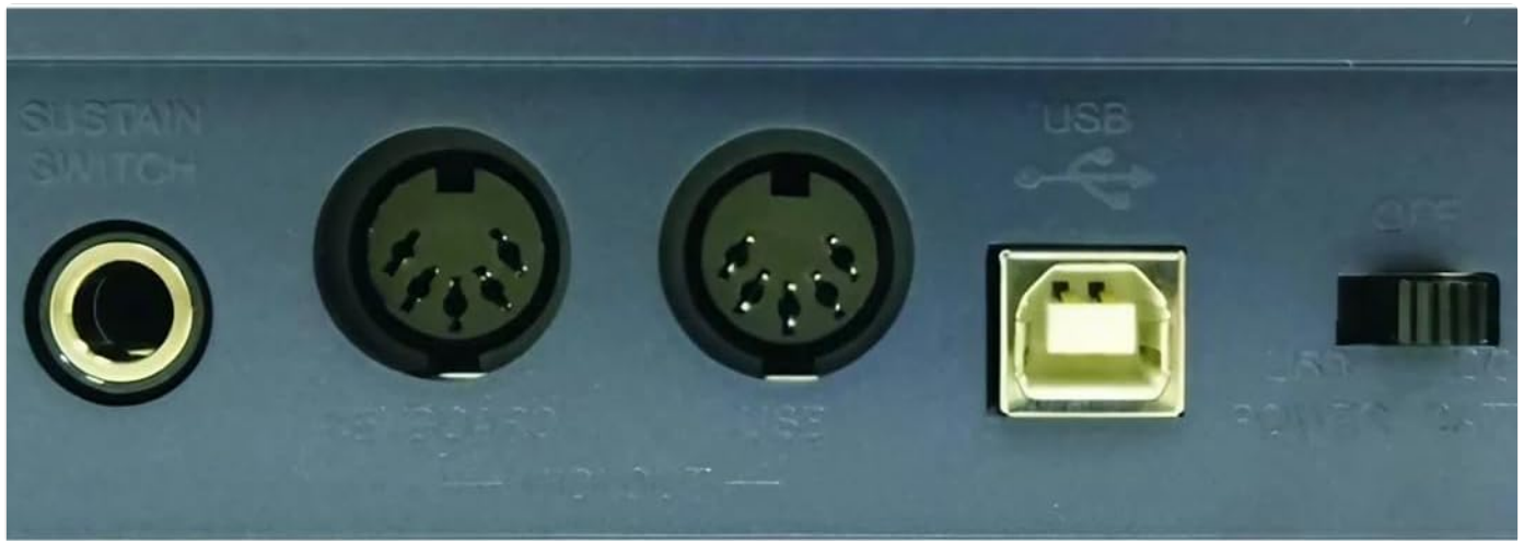
Figure 4.4: Rear panel showing the Sustain Switch input, KEYBOARD MIDI OUT, USB port, and Power switch.
