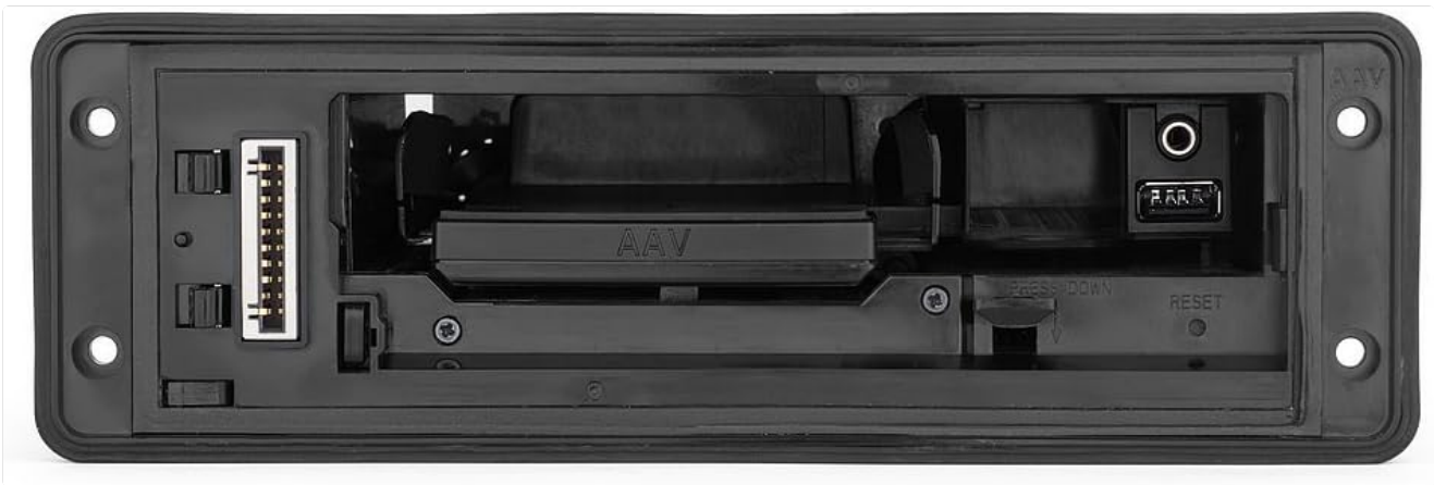
Image: The internal compartment of the stereo, revealing the USB port and 3.5mm auxiliary input.
