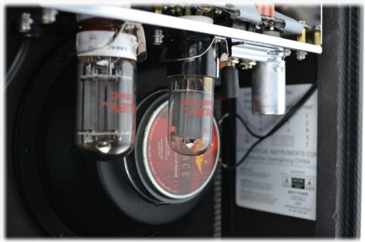
Figure 4.4: Internal view of the amplifier, showcasing the vacuum tubes and the Celestion speaker. The 12AX7 preamp tube, 6V6GT power tube, and 5AR4 rectifier tube are visible.
