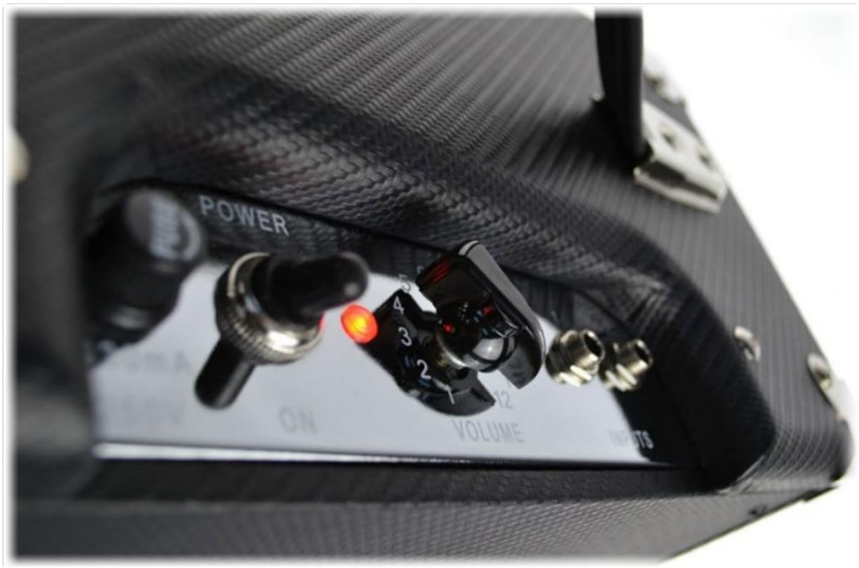
Figure 4.2: Close-up view of the amplifier's front panel controls. Visible controls include the Power switch, Volume knob, and Input jacks.
