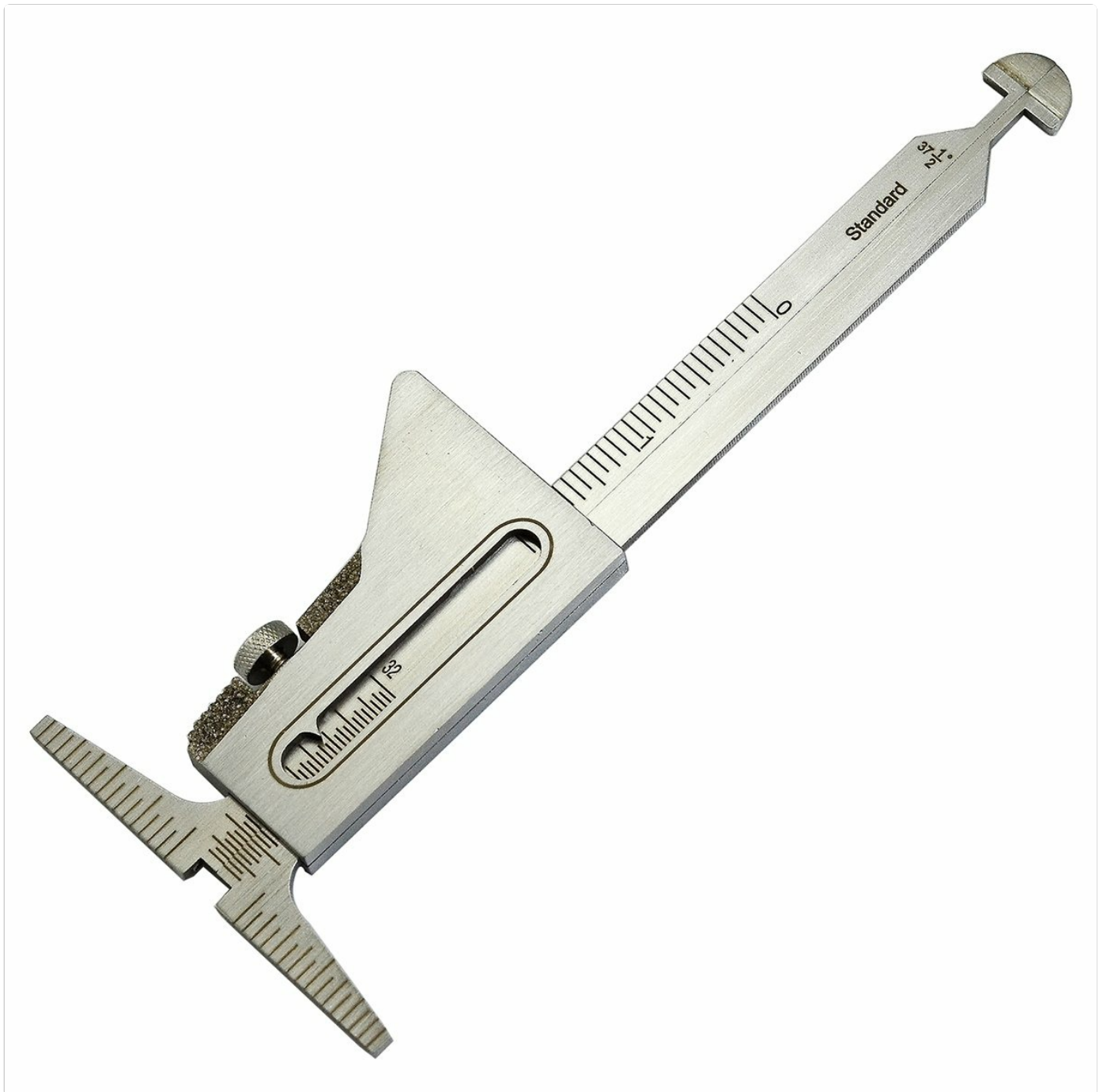
Figure 2: The gauge displaying both imperial and metric scales.
