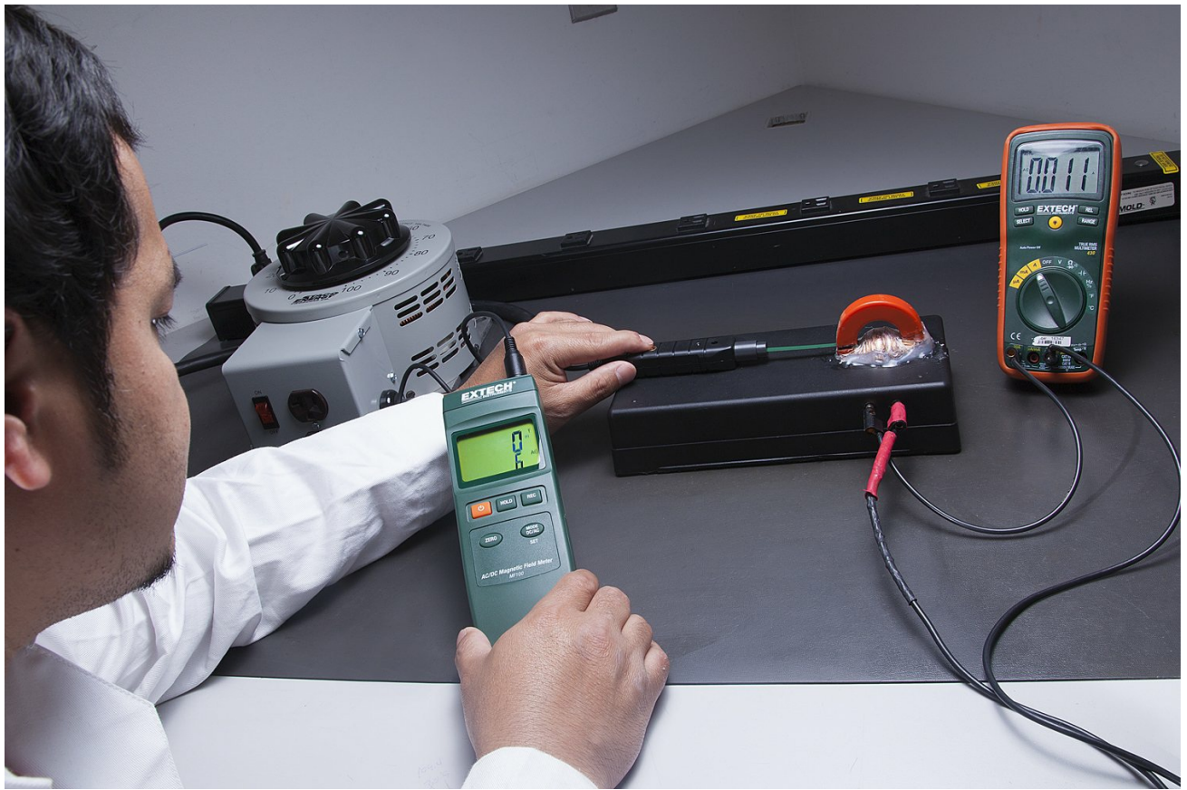
Figure 2: The Extech MF100 being used by a technician to measure a magnetic field in a laboratory environment.
