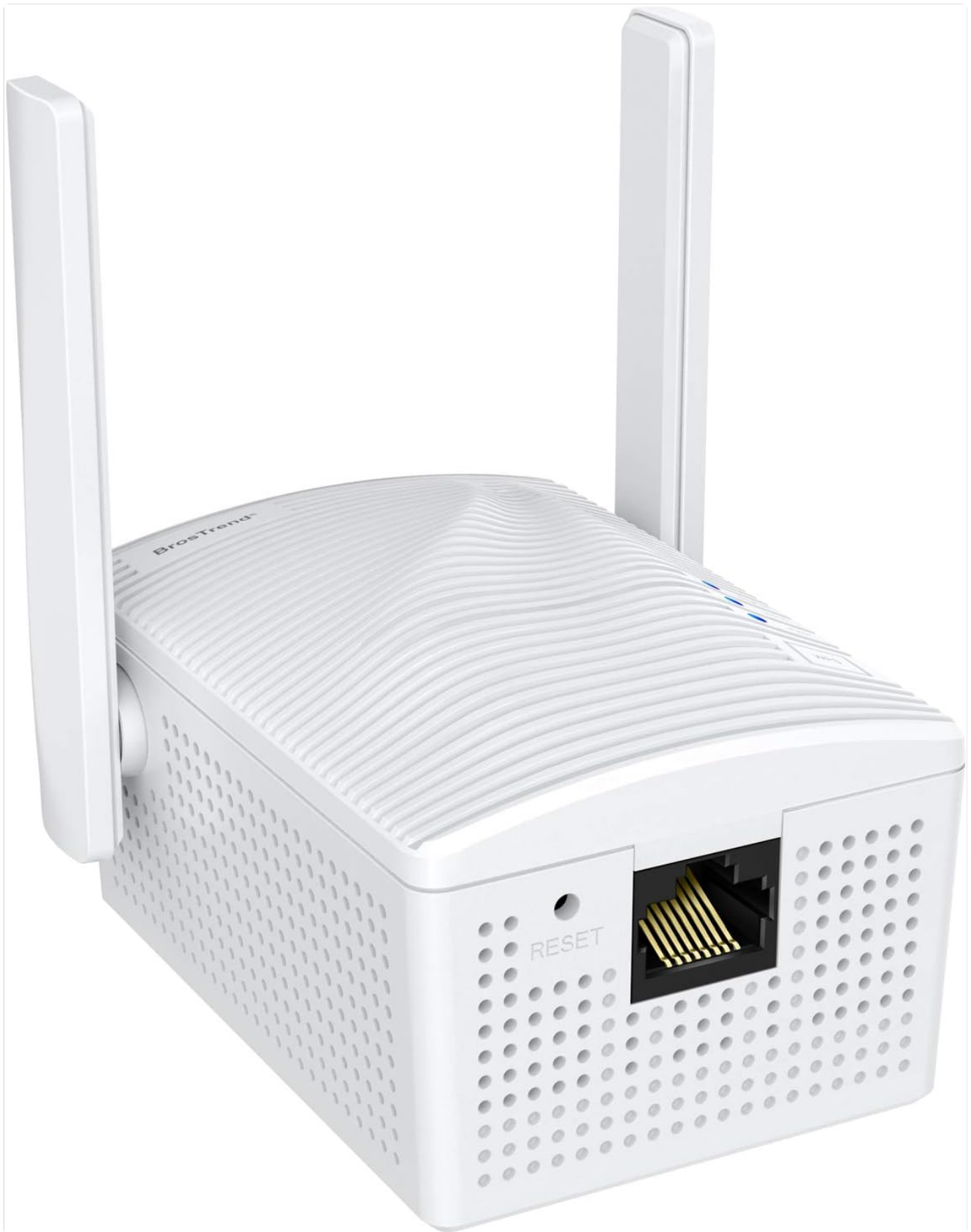
Figure 1: BrosTrend AC1200 WiFi to Ethernet Adapter with adjustable antennas and Ethernet port.
