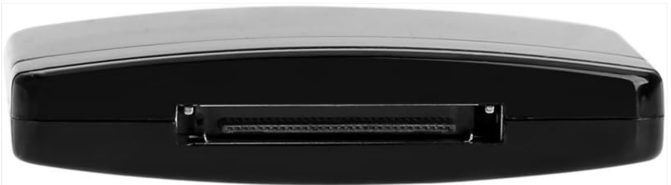
Image: The 30-pin connector on the Andoer Bluetooth receiver adapter. Ensure proper alignment when inserting into your speaker dock.
