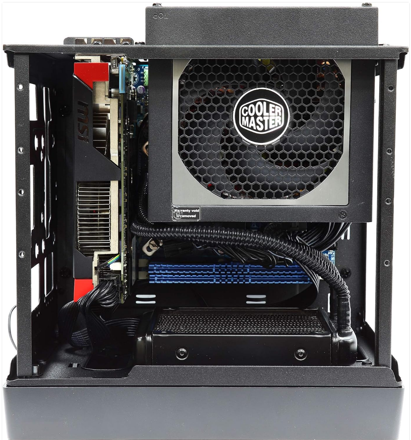
Figure 4.2: The Cooler Master V550 with all modular cables connected. This view demonstrates how the cables attach to the power supply, showcasing the fully modular design that allows for clean cable management.
