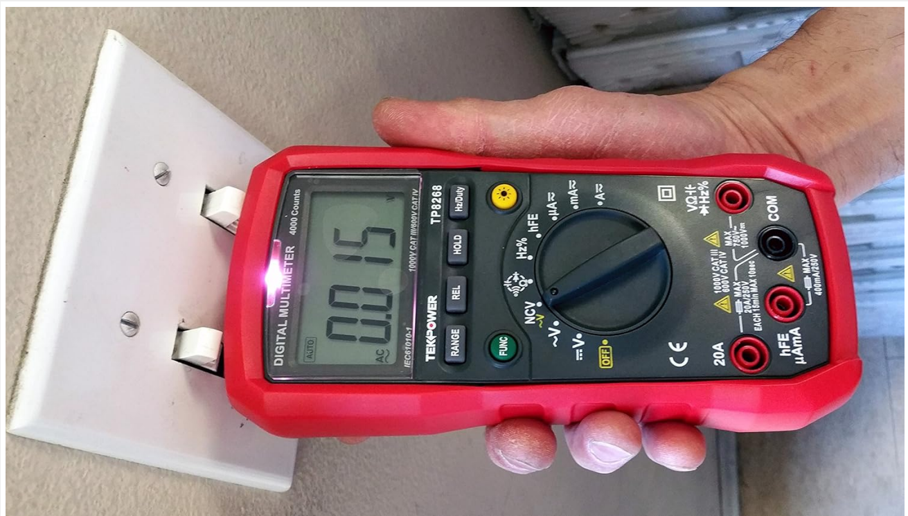
Figure 5: Performing a Non-Contact Voltage (NCV) test on a wall outlet with the Tekpower TP8268. This feature helps detect live AC voltage without direct contact.
