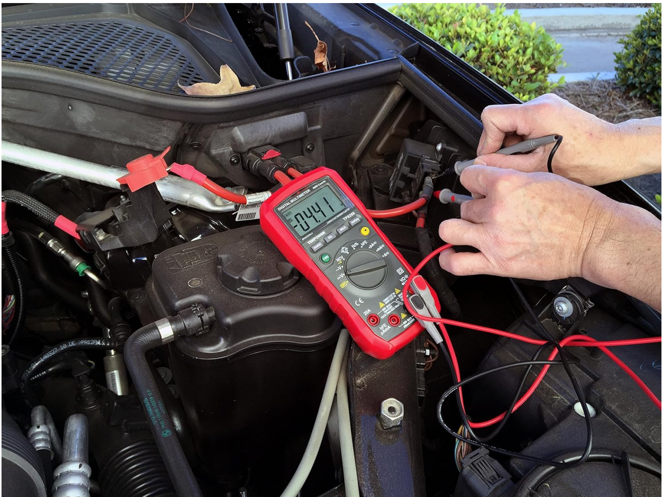
Figure 4: The Tekpower TP8268 in use, measuring voltage in an automotive engine bay. Always ensure proper lead connection and function selection.
