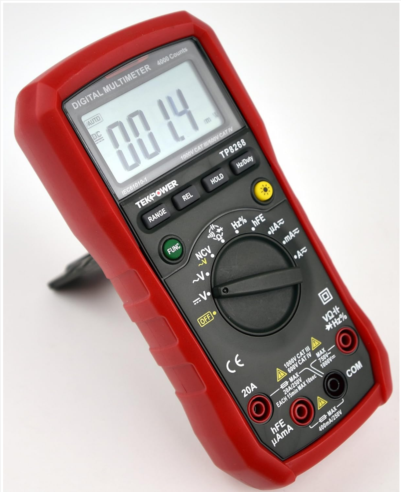
Figure 2: Front view of the Tekpower TP8268 Digital Multimeter, highlighting the display, rotary switch, and function buttons.
