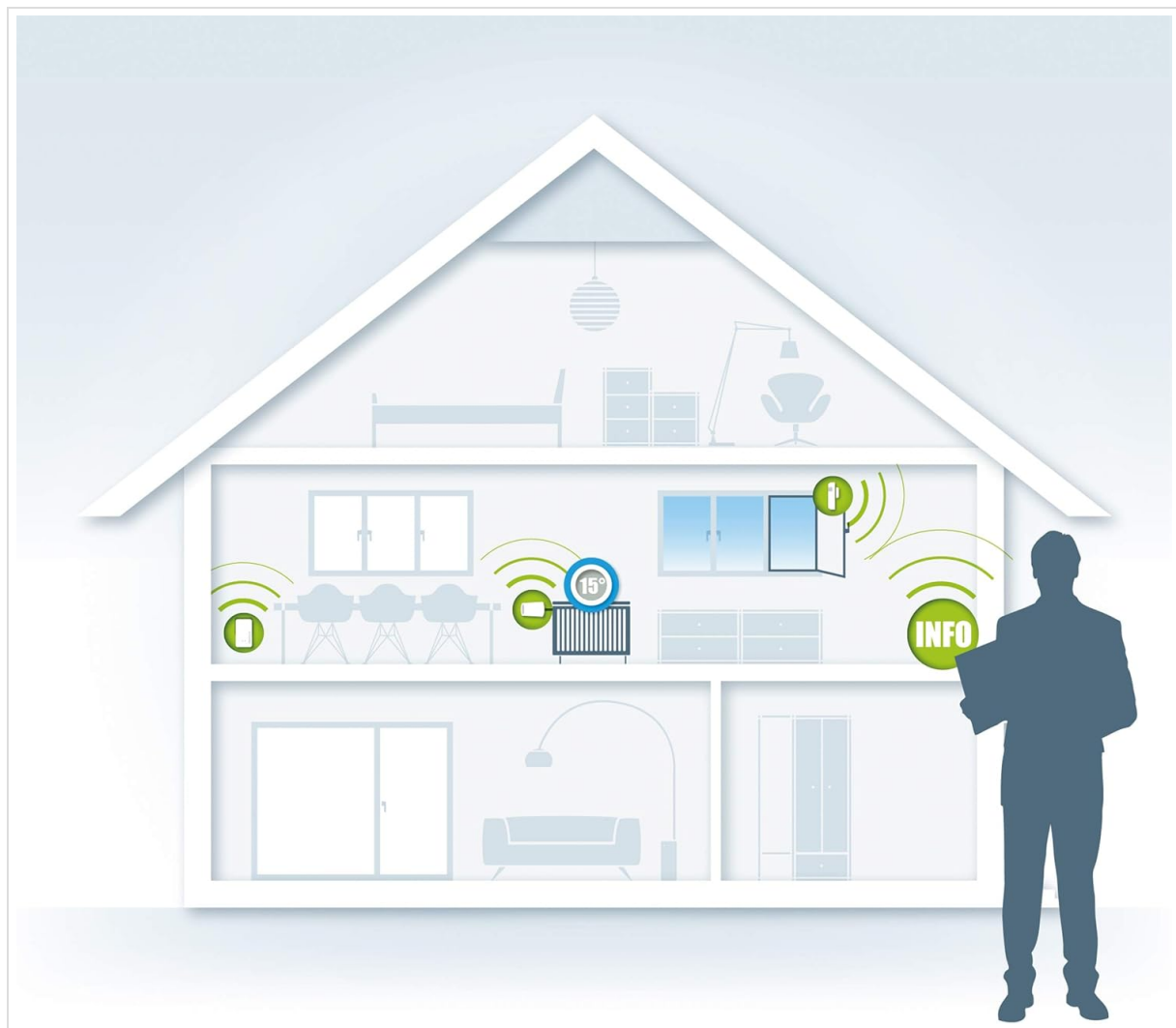
Image 3.3: An illustration of a smart home system indicating a window sensor detecting an open window, which can be used to automatically adjust heating.
