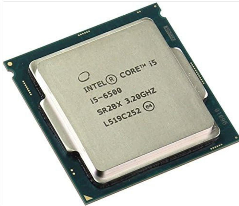
Figure 2: The Intel Core i5 6500 processor chip, showing the integrated heat spreader and pin array.
