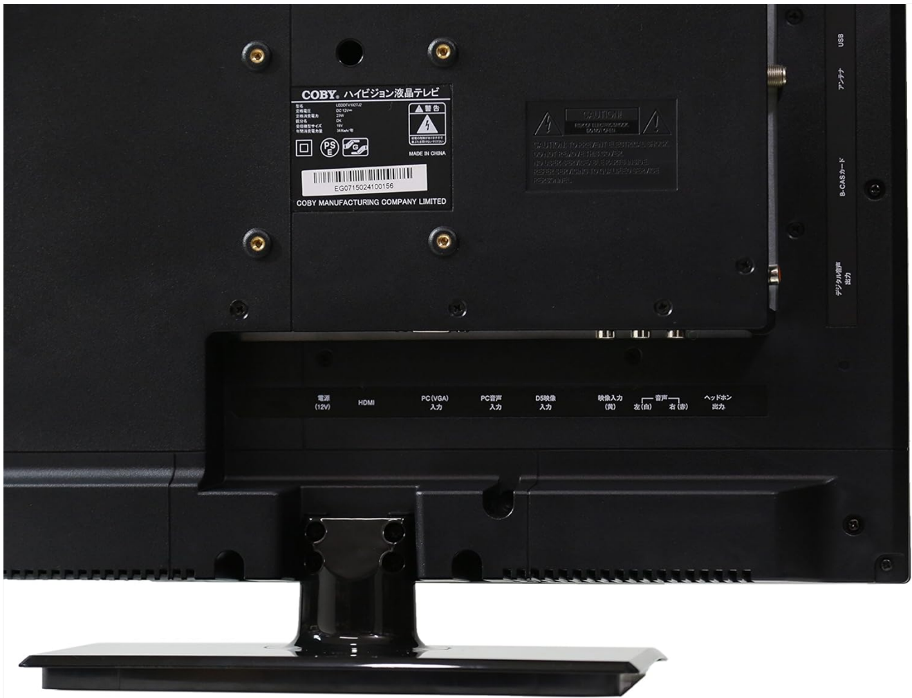
Image: Close-up of the rear panel of the Coby TV, showing HDMI, PC (VGA), USB, and antenna input ports.
