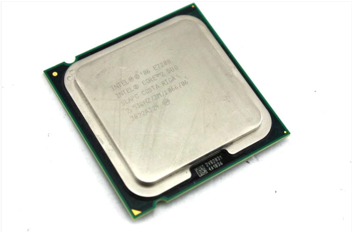
Image 1: Top view of the Intel Core 2 Duo CPU SLAPC processor, showing the integrated heat spreader with Intel branding and model information.
