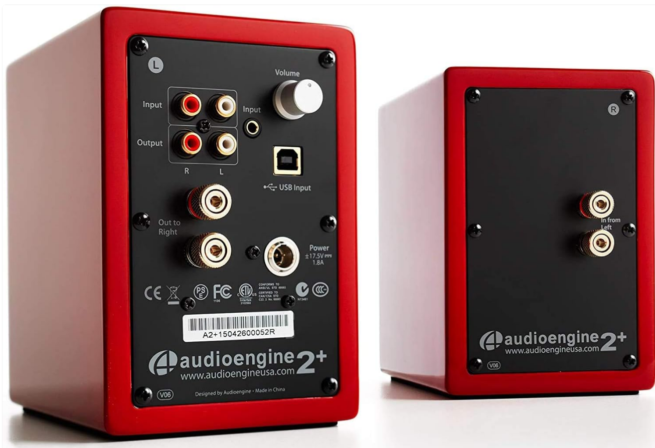
Image: Rear panel of the active speaker, highlighting various input and output connections.
