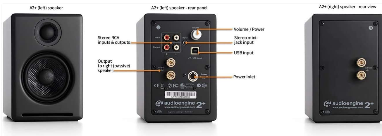
Image: A detailed diagram of the A2+ speaker connections, including volume, inputs, and outputs.
