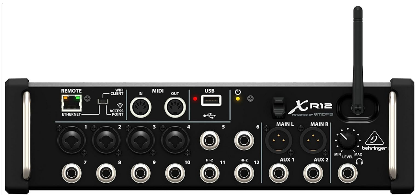
Image: Rear panel of the Behringer X Air XR12, showing all input and output connections, including XLR/TRS combo jacks, RCA inputs, MIDI I/O, USB, Ethernet, and Wi-Fi antenna.
