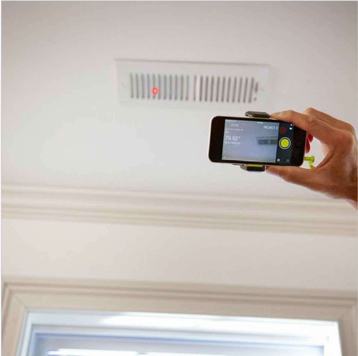
Image: A smartphone with the Ryobi ES2000 Infrared Thermometer attached, showing the app interface with temperature readings and a laser target.
