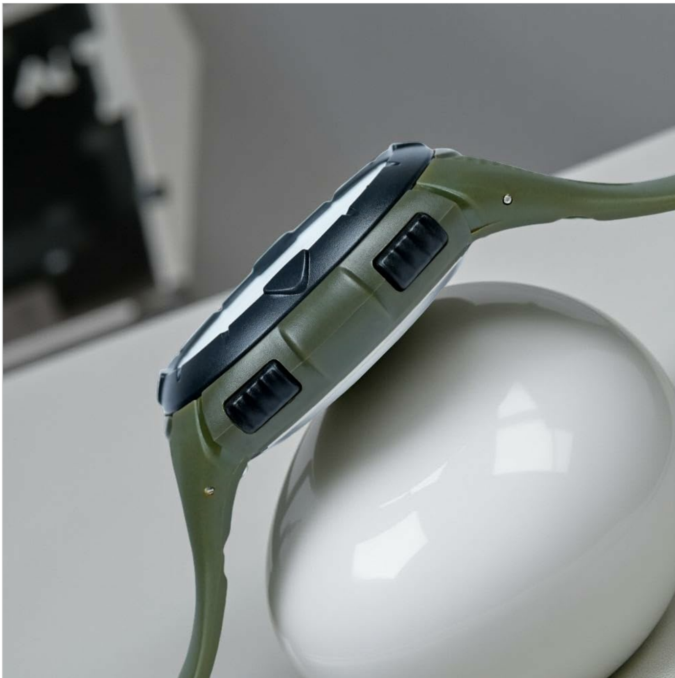
Image 3.1: Side view of the watch, illustrating the placement of the four function buttons.
