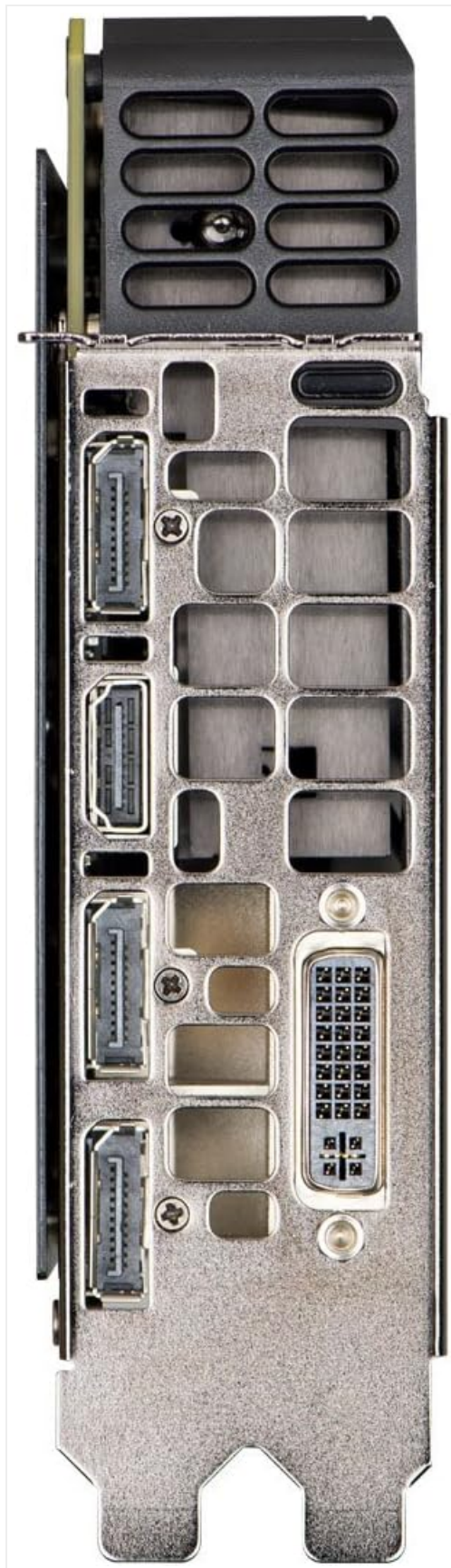
Figure 6.1: Rear panel showing the DVI, HDMI, and DisplayPort outputs.
