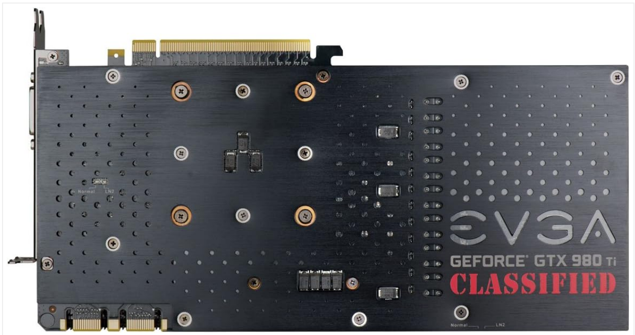
Figure 5.2: Rear view of the graphics card, highlighting the backplate and power connector locations.
