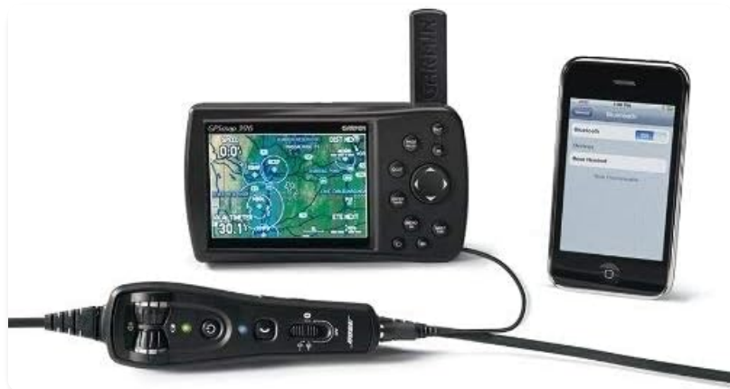
Figure 4: The control module of the Bose A20 headset, showing connectivity options.
