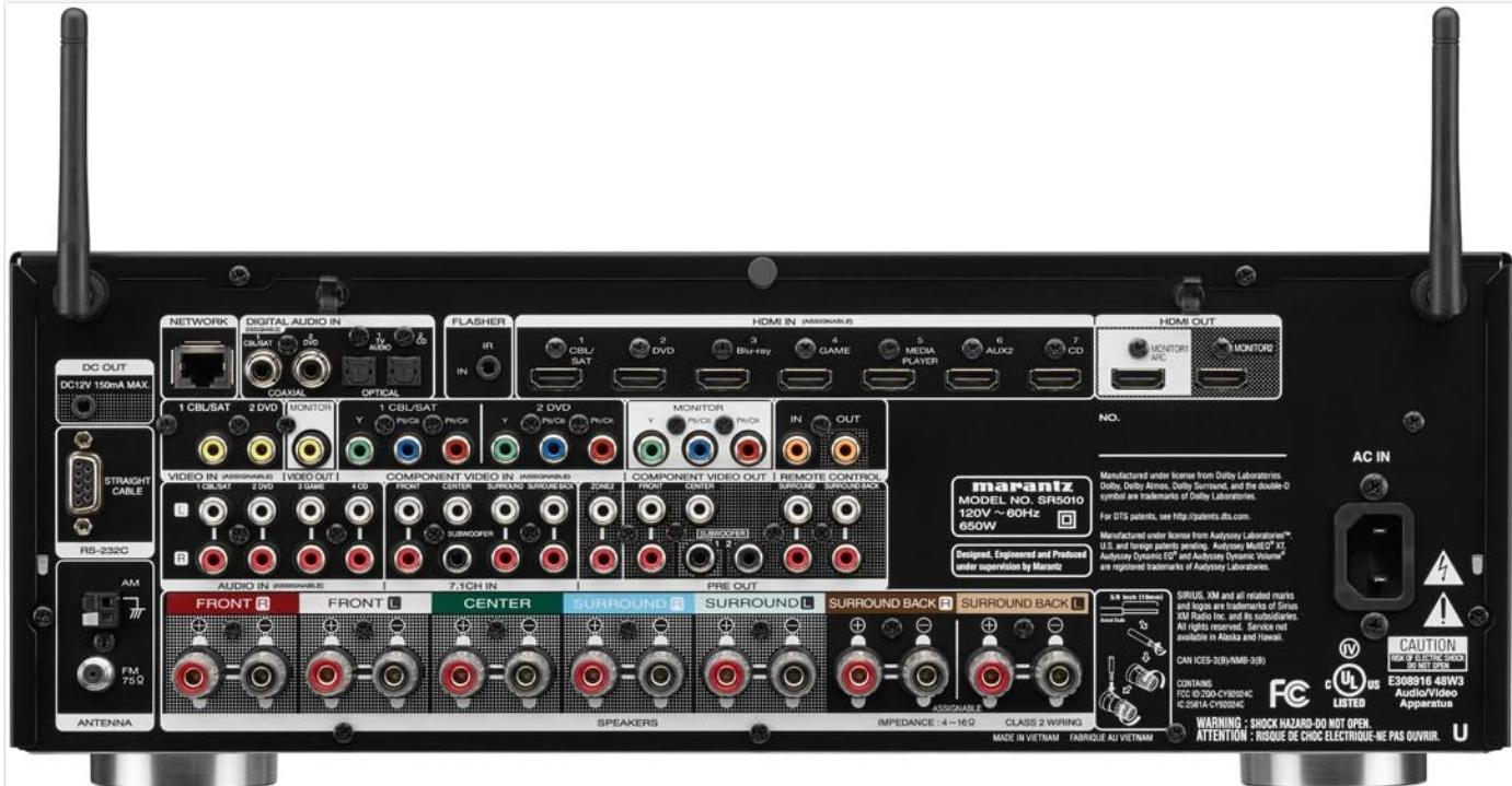
This image shows the rear panel of the Marantz SR5010 receiver, detailing the extensive array of connection ports. These include multiple HDMI inputs and outputs, digital audio inputs (optical and coaxial), analog audio inputs, component video inputs, speaker terminals for 7.2 channels, pre-out connections, Ethernet port, and antenna connections for Wi-Fi, Bluetooth, AM, and FM.
