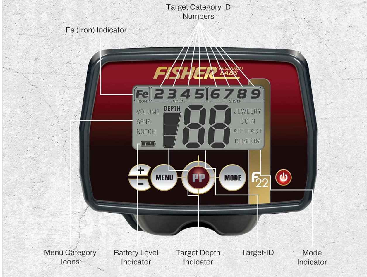
Figure 2: Close-up of the Fisher F22 control panel, showing the LCD screen and various control buttons.
