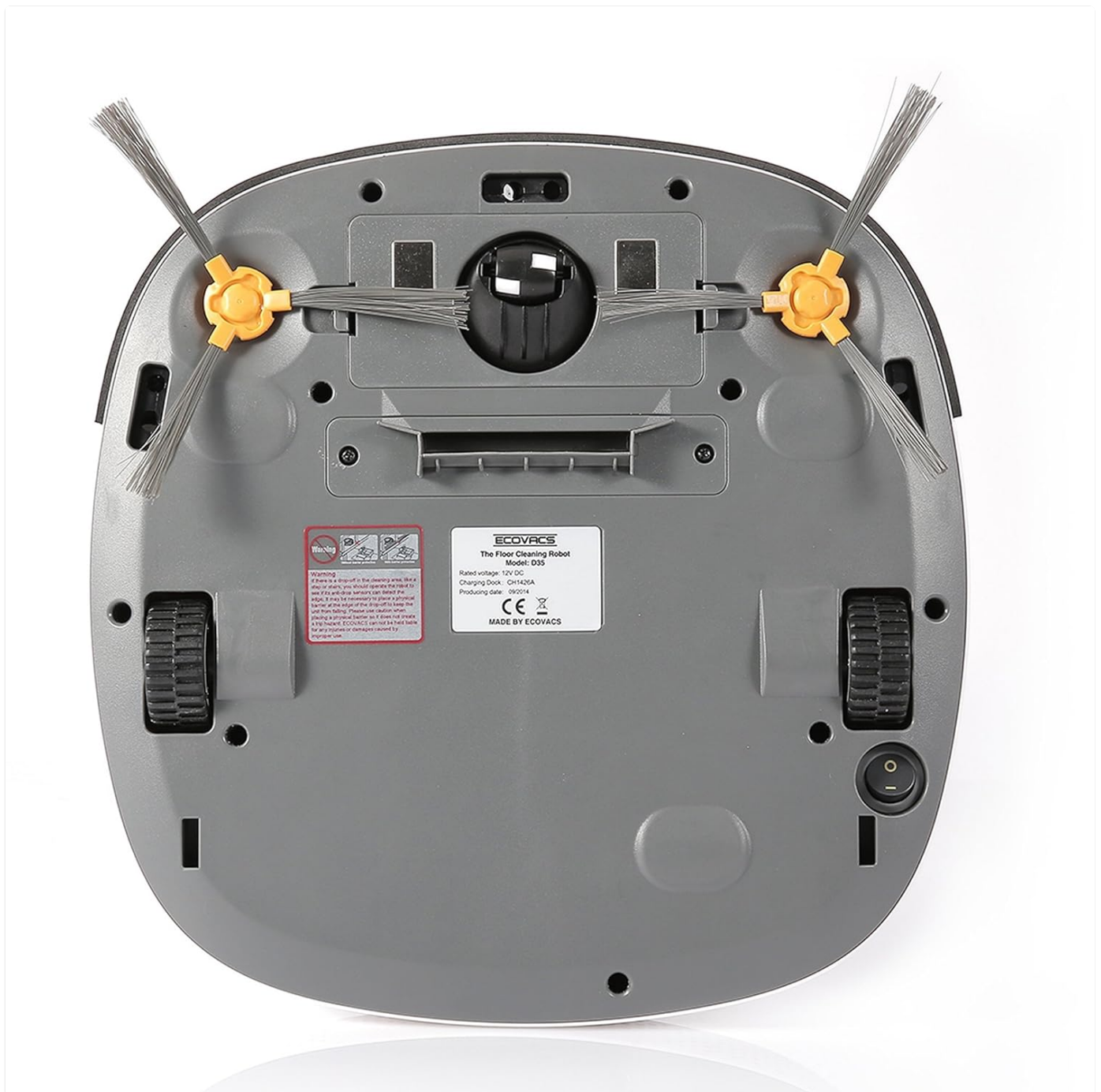
Figure 2: Bottom view of the DEEBOT D35, illustrating the side brushes, drive wheels, and suction inlet.
