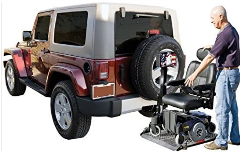
Figure 4: An individual carefully maneuvering a powerchair onto the Harmar AL500 lift, which is attached to the rear of a Jeep. This illustrates the loading process.
