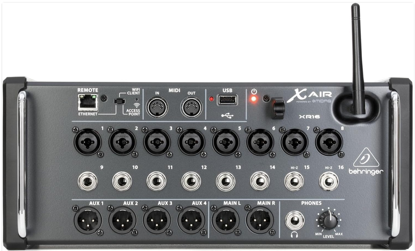
Figure 1: Top view of the XR16 showing the various input and output ports, including XLR/TRS combo jacks, auxiliary outputs, main outputs, MIDI I/O, USB port, and Ethernet port.
